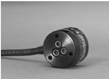
(a) Nano 17 van ATI Industrial Automation ( \phi 17mm x 14.5mm) [86].
