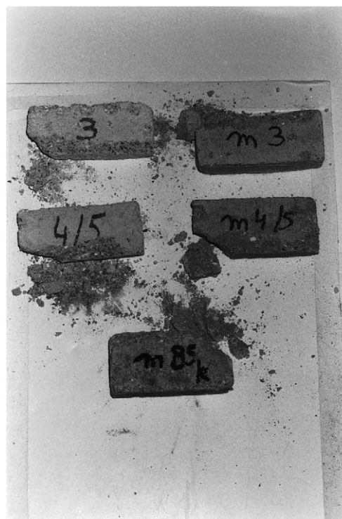
Fig. 5. Photograph of the test objects damaged and destroyed in the simulation of a high frost regime with a medium water content.
