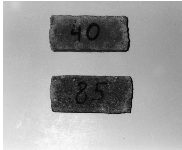
Fig. 7. Photograph of the test objects undamaged in the simulation of a high frost regime with a high water content.
