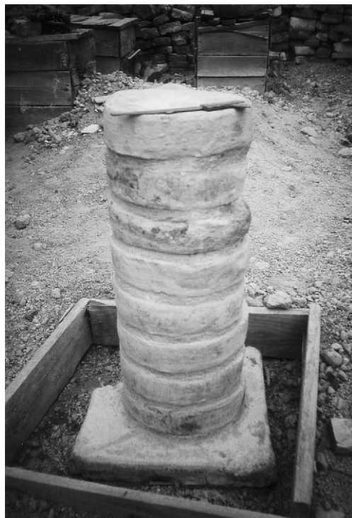
Fig. 8. Restoration mortar mix VO-1, undamaged after two winter seasons.
