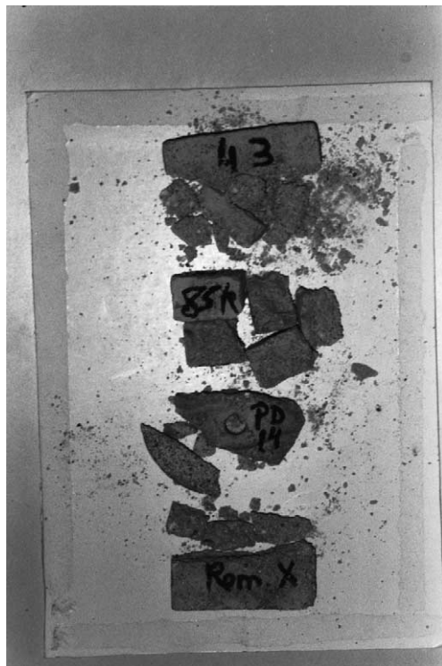
Fig. 6. Photograph of the test objects damaged and destroyed in the simulation of a high frost regime with a high water content.
