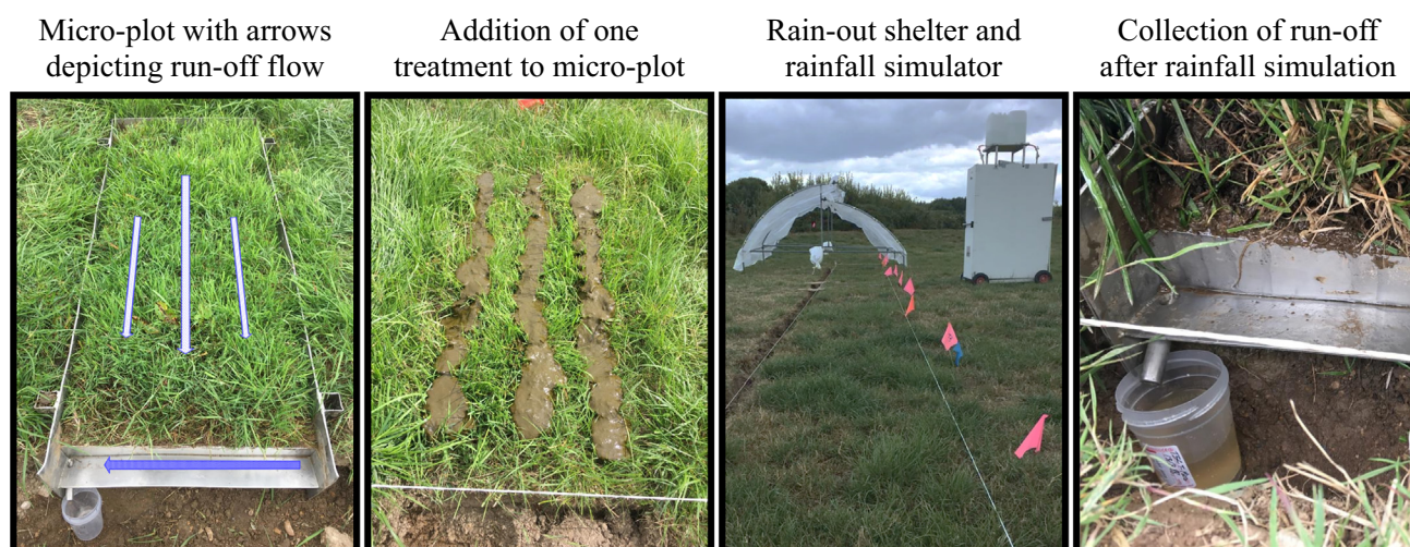
Fig. 1. Depiction of experimental set-up, using micro-plots (40 × 90 cm) to which different treatments (slurry or digestate) were applied before plots were subjected to a number of rainfall simulation events, where specialized frames allowed collection of runoff water.
