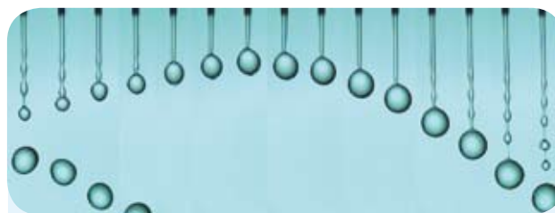
Fig. 1: Highspeed imaging of the ‘gobbling drop’ effect during the jetting from a 150 \mu m nozzle, caused by traces of polyacrylamid in aqueous solution at a critical flow rate at which the end drop will not detach, but climb up the liquid filament and consume (‘gobble’) several of the following drops (images acquired with 4000 frames per second).
