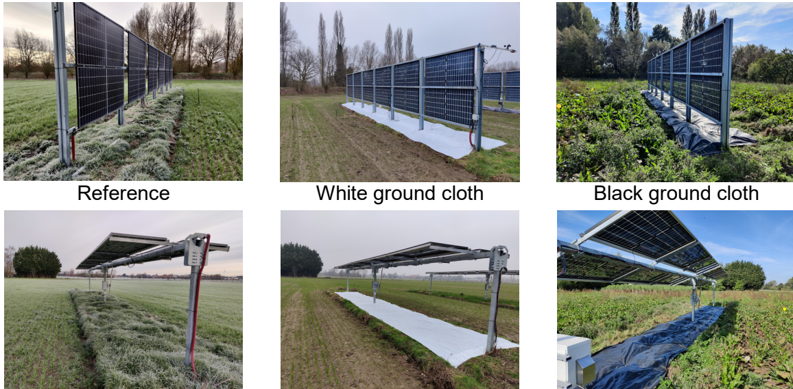
Figure 2: Overview of the different ground covers installed underneath the agrivoltaic systems.
