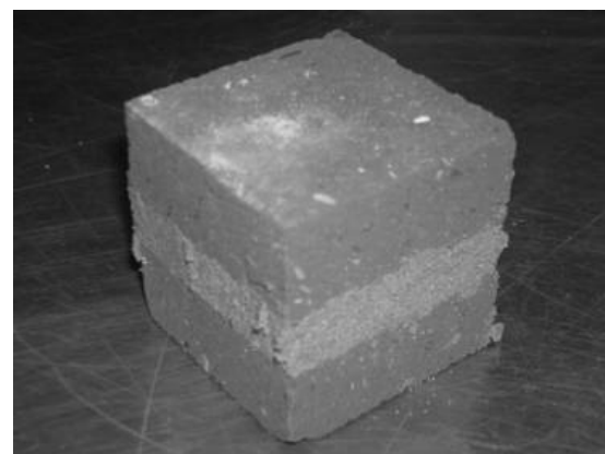
Step 4: sample before core drilling
