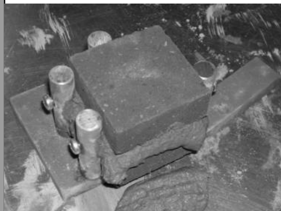
Step 3: parallel brick top layer
