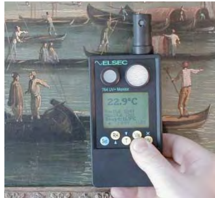
An Elsec data logger used to quantify the light received by an artefact.
