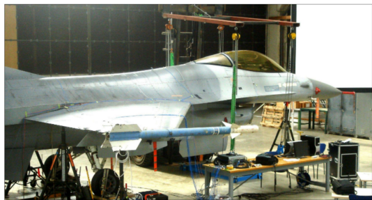
Figure 1: F-16 ground vibration test.
