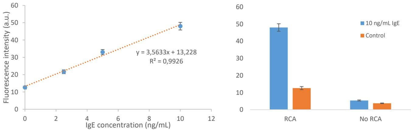
Figure 3. Calibration curve obtained after performing RCA creating multiple binding sites for the oligo label (left). Comparison of fluorescent signal obtained labelling with a single DNA oligo (reference) and using RCA (right). The reference signal was established using the same model assay except labelling with a single DNA oligo label. The error bars represent one standard deviation ( $n=4$ ).
