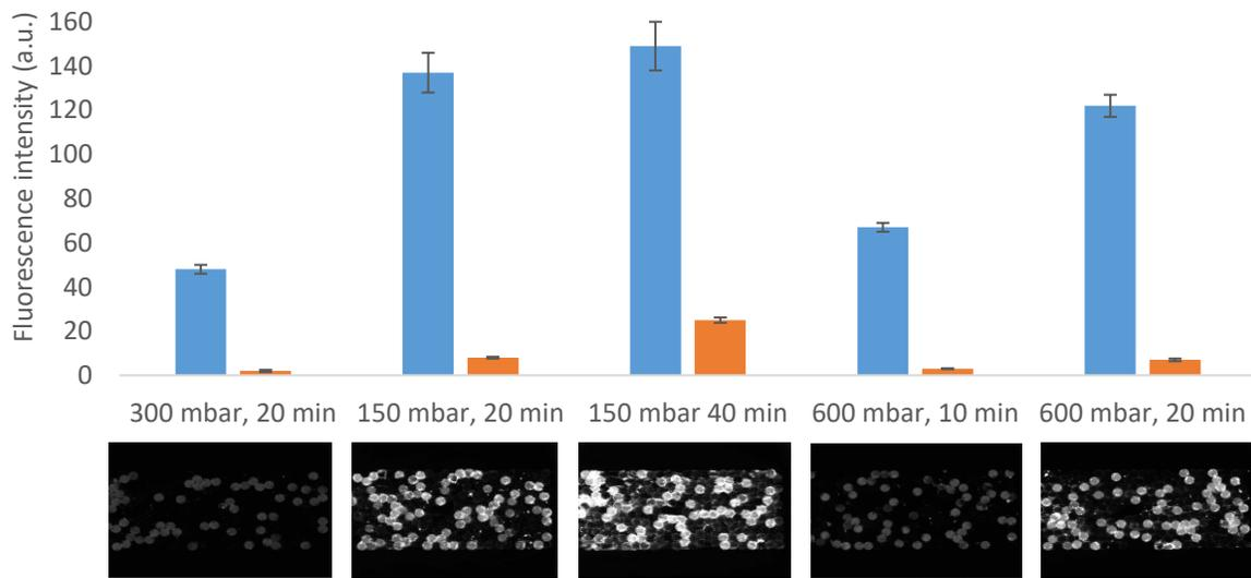
Figure 2. Rolling circle amplification for different flow rates (expressed as the applied pressure over the channel) and different amplification times. The blue bars represent signal obtained performing RCA on top of microparticles functionalized with the biotinylated secondary antibody. The orange bars represent the control particles. The error bars represent one standard deviation ( $n=4$ ).
