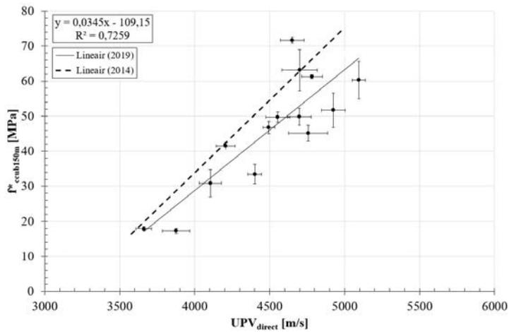
Figure 2. Correlation  $f^*_{ccub150m}$ -ultrasonic pulse velocity
