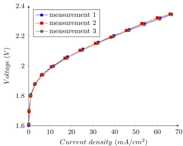
Fig. 9. Alkaline electrolyser polarisation curve
