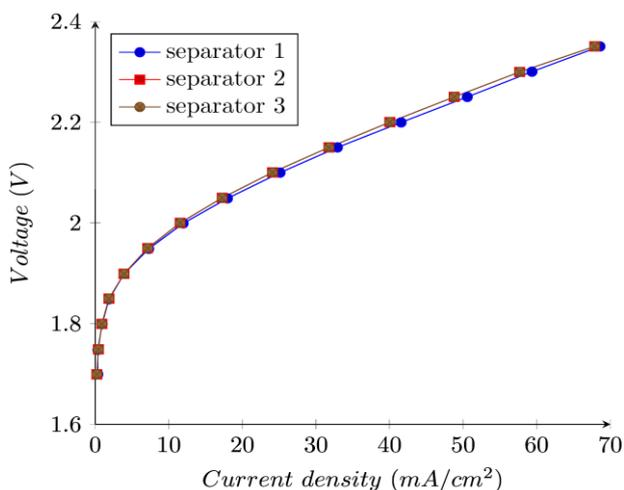
Fig. 10. Polarisation curve after interchanging the separator
