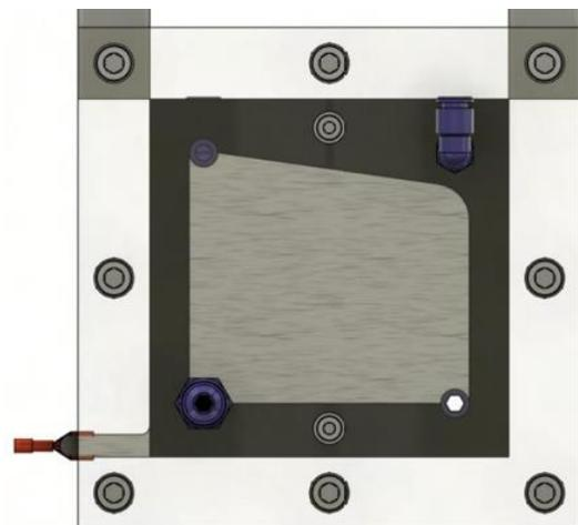
Fig. 6. Electrolyser cross-section at the spacer level
