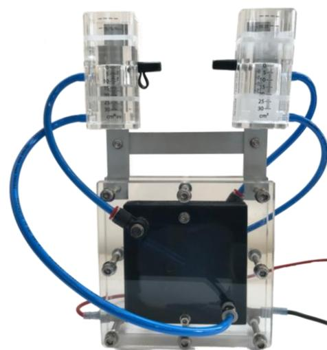
Fig. 8. Fully assembled electrolyser
