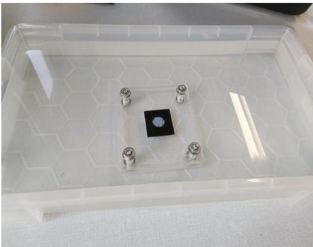
Fig. 5. Submerged gaskets test
