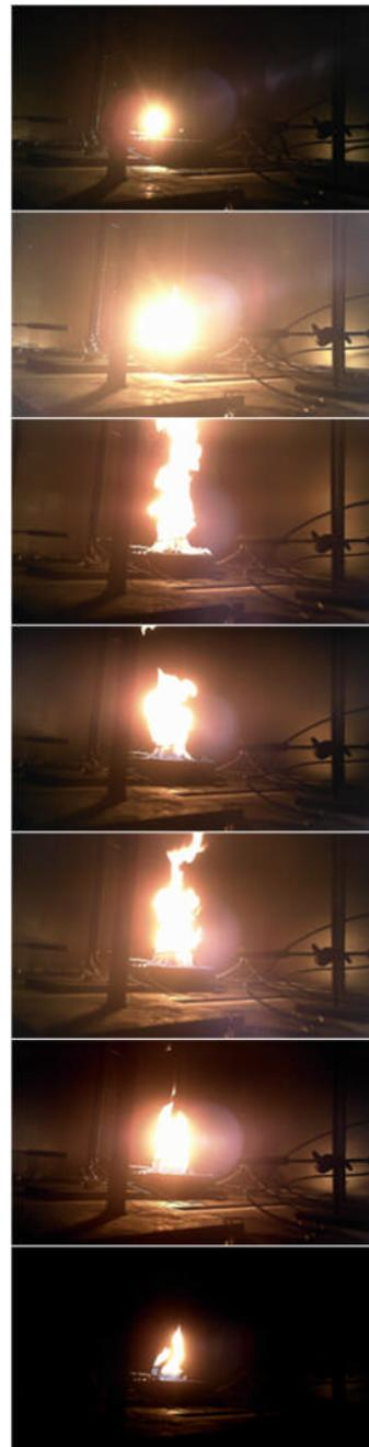
Fig. 1. Sequence of images during a NYX fire test of [21]. Pictures by H. Prêtre – IRSN. From top to bottom: ignition of pilot flame; ignition of fire source; steady combustion (3 pictures); decay phase; extinction.
