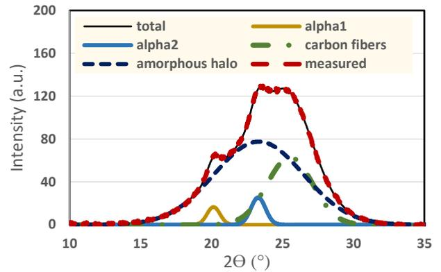
Fig. 3. Typical XRD pattern of the CF/PA6 sample with peak-fitted peaks.
