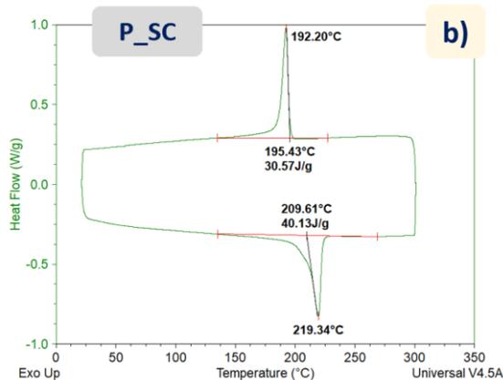
Fig. 2. DSC curves for CF/PA6 composites processed at different cooling rates: (a) F\_WC, (b) P\_SC.
