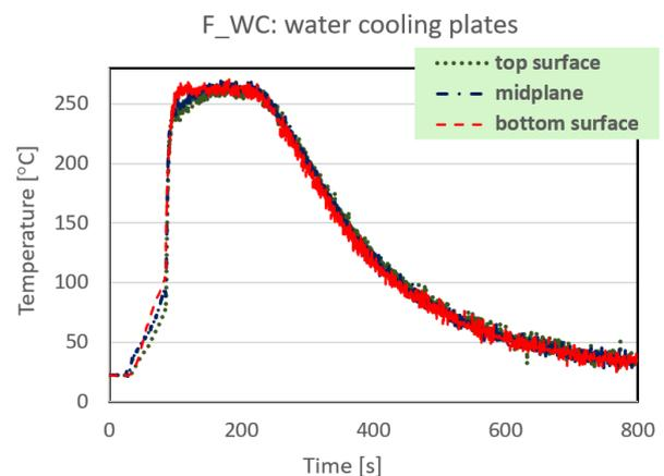
Fig. 1. Thermal history of the manufacturing process of F\_WC plate recorded at three surfaces of the laminate.
