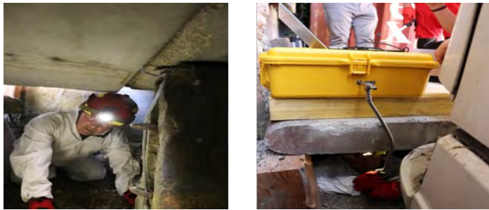
Figure 1. Testing of the RESCUE-MIMS in the field under the scenario “People Trapped Under the Rubbles” that took place in Limoges, France in cooperation with the PUI team
