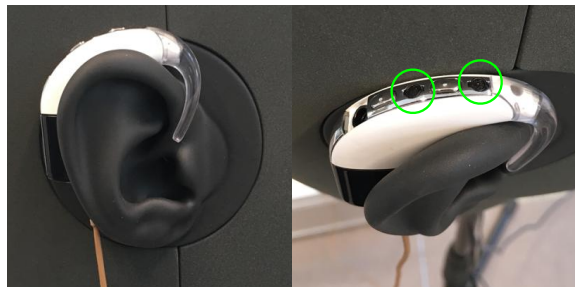
Figure 2: Dummy BTE pieces used for creating the database. Each BTE piece consists of two omnidirectional microphones as indicated by the circles.
