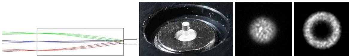
Figure 24. The telescope pupil is projected on the fibre input end, by means of a gradient index lens of pitch 0.25. The last two images show the far field patterns at the output of the octagonal fibre in narrow band. Fields: 0, 0 (left) and -1, 0.
