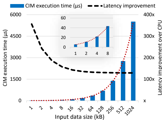
Fig. 7: Execution time to encrypt different input text sizes and the improvement achieved compared to the software implementation
