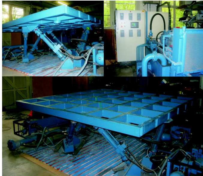
FIGURE 7.1: Electro-hydraulic shaker; top left: cylinders in Stewart configuration; top right: hydraulic group and numerical controllers; bottom: platform
