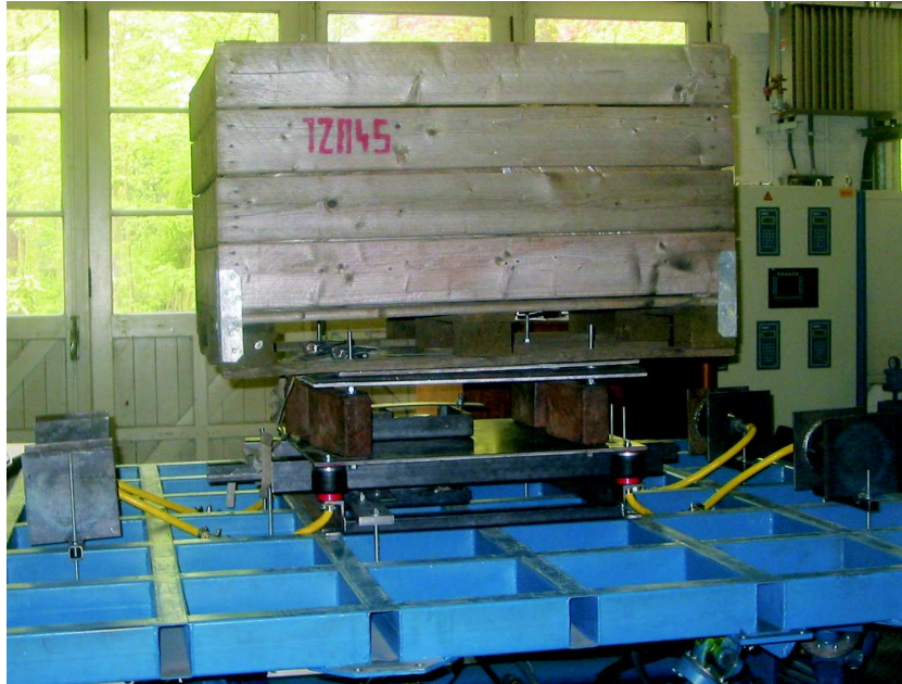
FIGURE 7.6: Evaluation setup containing suspension system loaded with a mass resembling a real cabin
