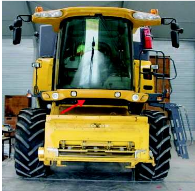
FIGURE 3.5: Placement of the L-shaped measuring device on the supporting structure of the cabin, indicated by the arrow
