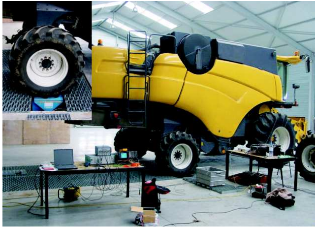
FIGURE 3.13: Setup for evaluation of the rubber mounts by excitement under rear tire of the combine
