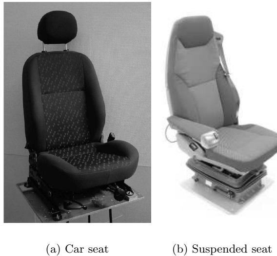
FIGURE 2.7: Photograph of a conventional car seat and a suspended seat for bus, tractor or truck
