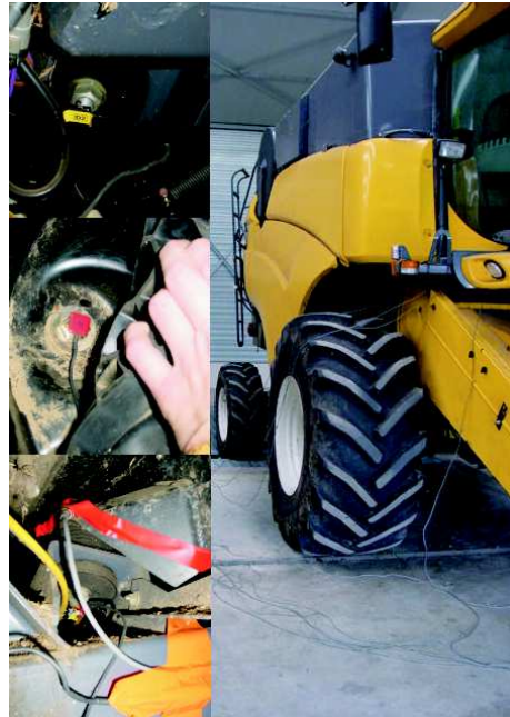
FIGURE 3.14: Placement of the accelerometers to determine the behavior of the rubber mounts
