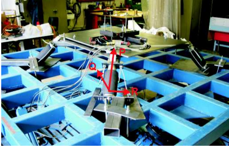
FIGURE 5.4: Spring suspension system with four Firestone Airmount 7012 springs put at a 45 degree angle with respect to the vertical direction [33] (P,Q and R indicate the principle axes for one spring)
