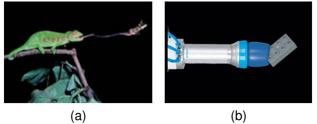
Fig. 1. Chameleon tongue and the related bio-inspired soft gripper [9]. (a) The flexible chameleon tongue that can adapt to the shape and size of a prey and firmly enclose the prey. (b) The investigated gripper inspired by the nature of the chameleon tongue.
