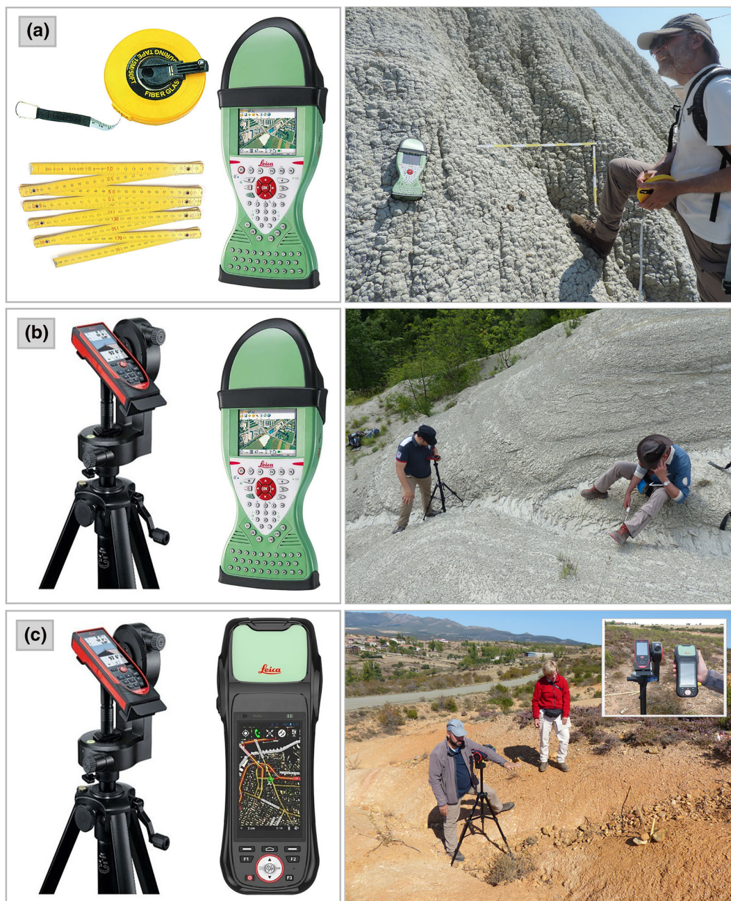
FIGURE 5 Instrumental settings used for the geometric and morphometric characterization of each selected gully head, in (a) the Leonina, (b) Verghereto, and (c) Guadalajara study areas.
