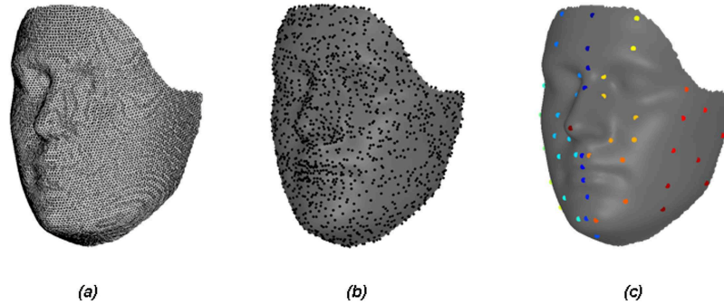
Figure 5.1: Illustration of the reference face, being the average face of the database. (a) The reference tessellation. (b) Shaded rendering with the points indicated used during non-rigid registration. (c) Same shaded rendering, with the 52 face landmarks indicated using a distinctive color for every landmark. This is shown to compare the landmark consistency registration results in figure 5.2(c) with the landmark positions of the reference face
