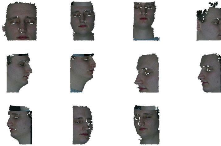
Figure 4.15: 11 patches of the real-live data set rendered with texture information. Note the bad texture alignments in some patches, due to a time-delay between texture and geometry image (e.g. figure 4.1(middle))acquisitions.
