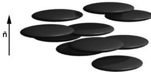
Figure 1.9: Schematic representation of the discotic nematic phase ( $N_D$ ).
