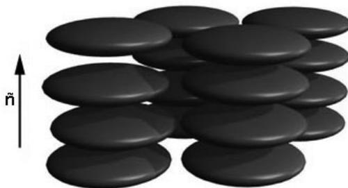
Figure 1.10: Schematic representation of a columnar phase.
