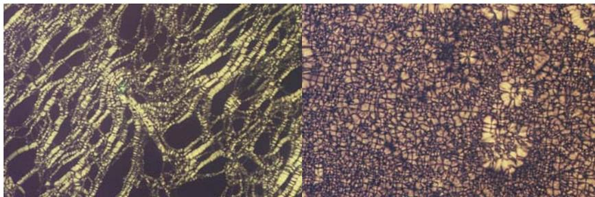
Figure 4.7: Left: oily streak texture of the SmA phase of  $[\text{Ru}(\text{bipy})_2\text{Lv}](\text{NTf}_2)_2$  at  $178\text{ }^\circ\text{C}$  ( $200\times$  magnification). Right: focal conic texture of the SmA phase of  $[\text{Ru}(\text{bipy})_2\text{Lv}](\text{NTf}_2)_2$  at  $165\text{ }^\circ\text{C}$  ( $200\times$  magnification).
