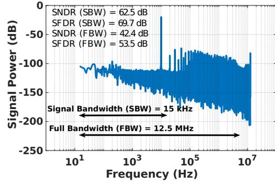
Fig. 5: 15000000-point FFT for a 10-kHz input sine.
