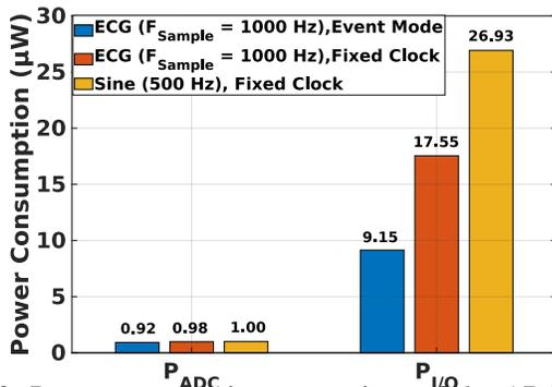
Fig. 9: Power consumption comparison of the ADC and I/O buffers for an ECG signal and a 500-Hz sine wave.
