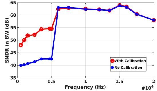
Fig. 6: SNDR in the 15-kHz signal band for different input frequencies.
