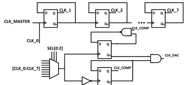
Fig. 3: Clock generator block of the LCADC.
