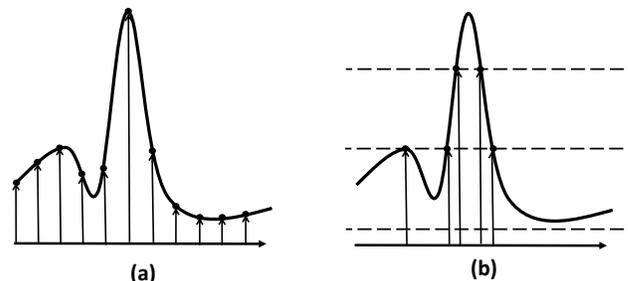
Fig. 1: (a) Regular Nyquist sampling and (b) event-driven level-crossing sampling.
