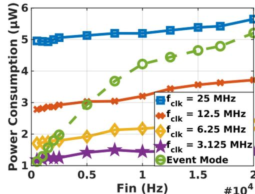
Fig. 7: Measured power consumption as a function of the sine wave input frequency in fixed and event-driven modes.
