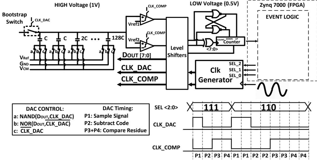
Fig. 2: Overview of the proposed level-crossing ADC and its timing diagram.
