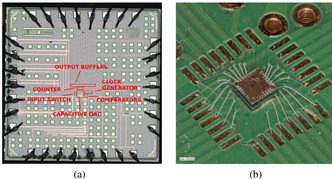
Fig. 4: (a) Die photograph and (b) chip bonded to PCB.
