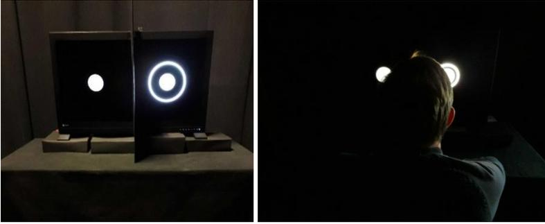
Figure 3.4: Pictures of the experiment set-up. (Left) A view of the experiment set-up showing the shield and the screen; the reference stimulus is displayed at the left half and the test stimulus at the right half. (Right) An observer during the adaptation period.
