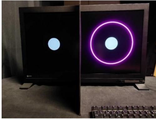
Figure 5.2: Experimental setup with an example of the reference scene and the test scene with a magenta ring.
