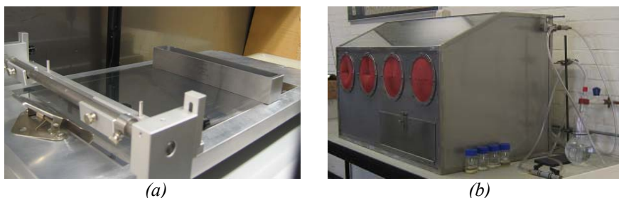
Figure 2.6: Setup used to synthesize polyethersulfone membranes: (a) the filmograph and (b) the membrane box, in which an atmosphere with controlled relative air humidity could be established
