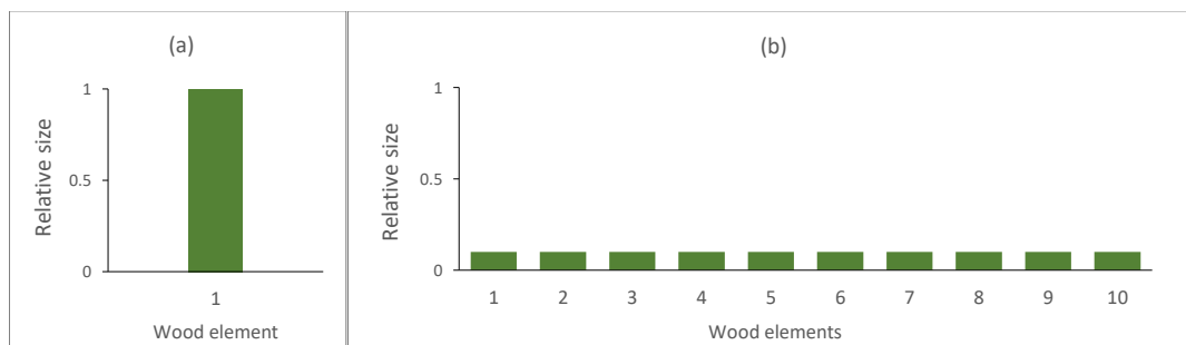
Figure 4.2: The size distribution pattern to support the conceptual explanation Relative size distribution in the flow containing only a plank (a) and when plank is broken down (b)
