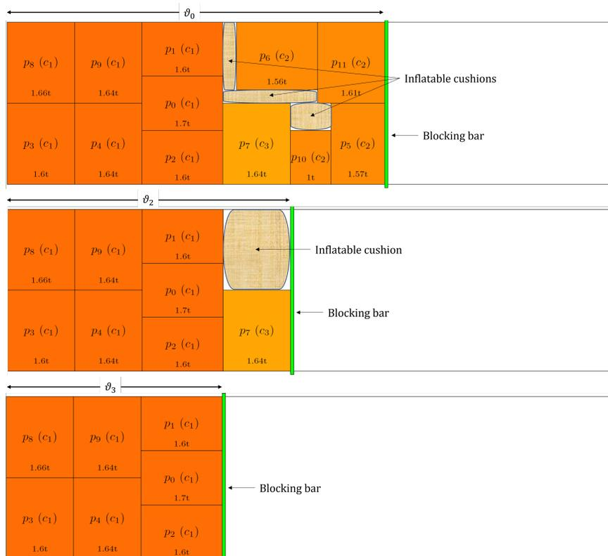
**Figure 3:** Securing pallets with a blocking bar and inflatable cushions. After unloading pallets, the bar is moved closer towards the front wall and any empty spaces behind the bar are filled with cushions.
