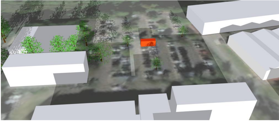
Fig. 9 The shadow pattern from surrounded obstacles around 10 a.m. on 21 Jan. 2020.
