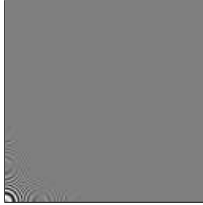
Figure 6.3: The zone plate function used for testing sampling patterns. This reference image was constructed by sampling the zone plate function using a stratified sampling pattern with one million samples per pixel. The image was reconstructed using a Mitchell filter of 4 \times 4 pixels.
