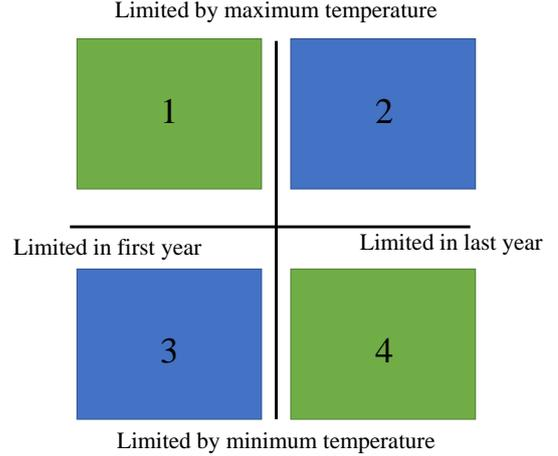
Figure 2: Graphical representation of the four groups of borefields.
