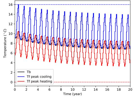
Figure 4: Example of a borefield, dominated by heat extraction and limited in the first year of the study period by the cooling load.
