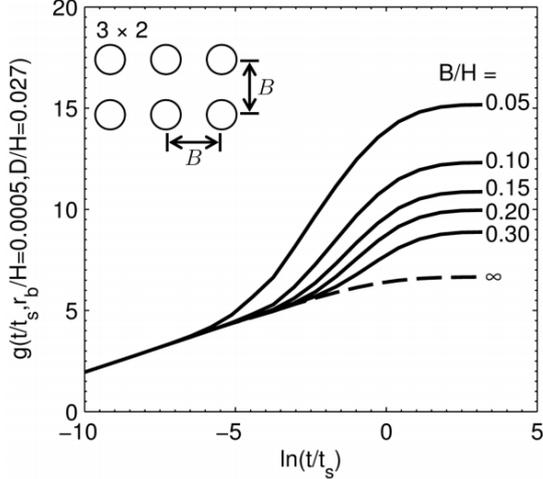
Figure 1: Example of  $g$ -functions for different configurations (Bernier, 2015). ( $B$  the borehole spacing,  $H$  the borehole depth,  $r_b$  the borehole radius,  $t_s$  a normalised time)
