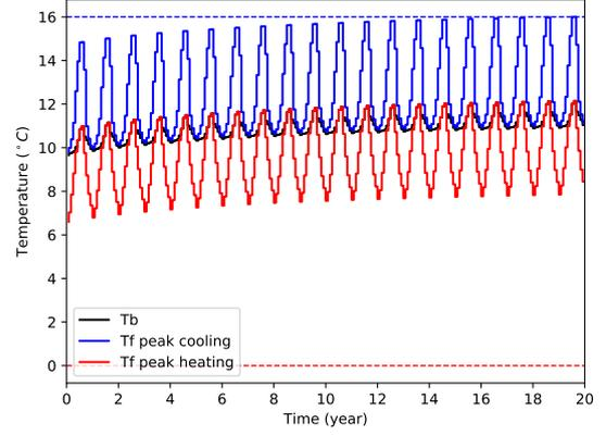
Figure 3: Example of a borefield, dominated by heat injection and limited in the last year of the study period by the cooling peak. ( $T_f$  is the mean fluid temperature)
