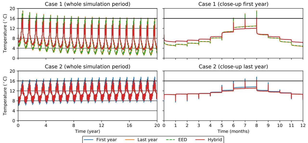
Figure 6: Dynamically simulated temperature profiles based on the borefield lengths derived from EED, FY, LY and the Hybrid method for Case 1 and 2.
