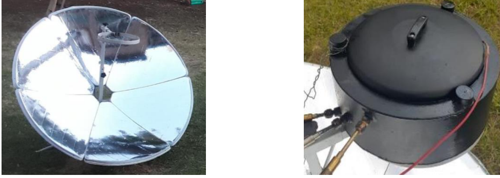
Fig. 1: Photograph of the parabolic dish solar cooker with TES system implemented in the cooking pot. Left: parabolic solar collector, right: cooking pot with TES system
