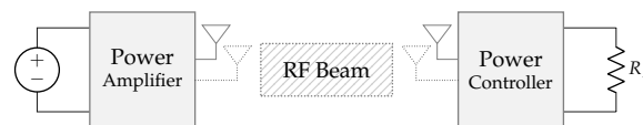
Figure 17. Schematic of an RFPT system. Antenna arrays (in dashed line) at the transmitter and/or receiver can be employed to increase the power transfer.
