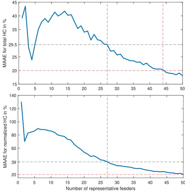
Fig. 4: MAAE of stochastic PV HC scaling from representative feeders using all features
