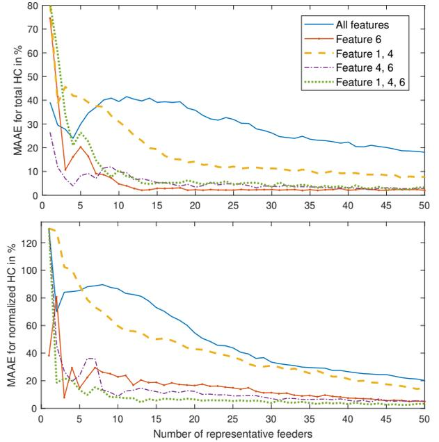
Fig. 5: MAAE of stochastic PV HC from representative feeders after feature reduction
