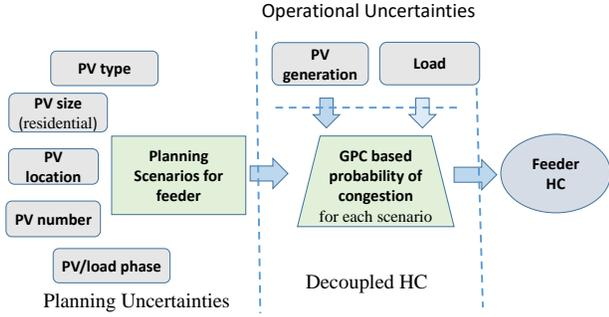
Fig. 1: Decoupling of planning and operational uncertainties to calculate PV HC [11]
