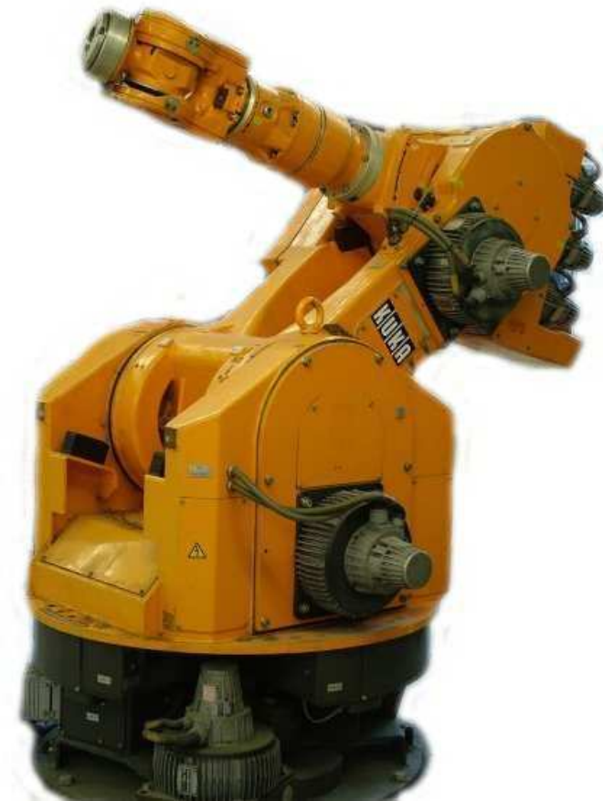
FIGURE 7.12: In the experimental setup the Kuka 160 six degree of freedom industrial robot is used.
