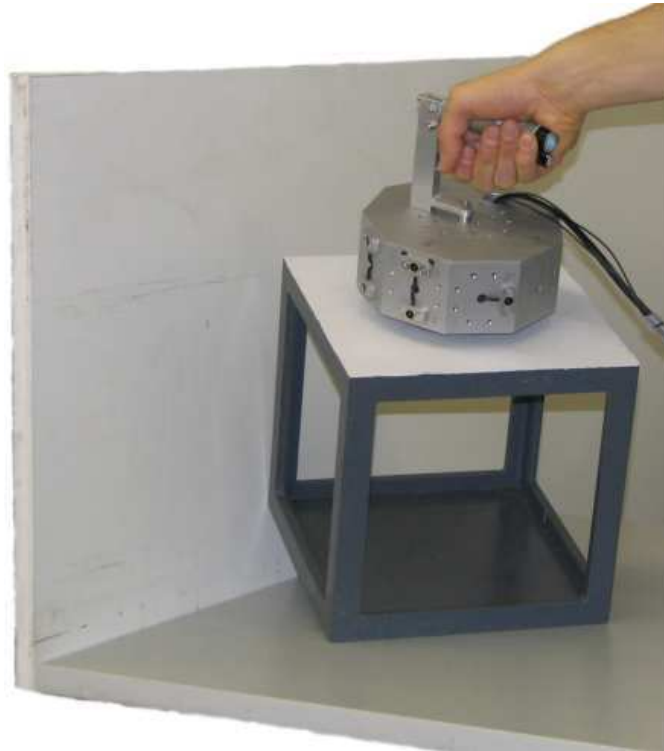
FIGURE 7.11: In the experiments to validate the presented approach a human demonstrator uses a demonstration tool to manipulate a cube in contact with three perpendicular faces.
