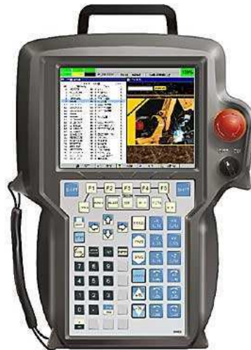
FIGURE 2.1: A modern teach pendant equipped with an LCD screen is used to manually move an industrial robot in joint or Cartesian space.
