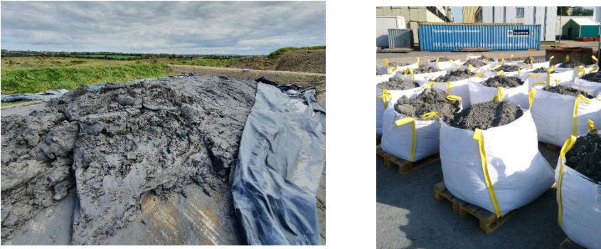
Figure 1: Freshly sourced tailings from the storage facility at Boliden Tara (left) and sun-dried tailings in big bags at Thyssenkrupp (right).
