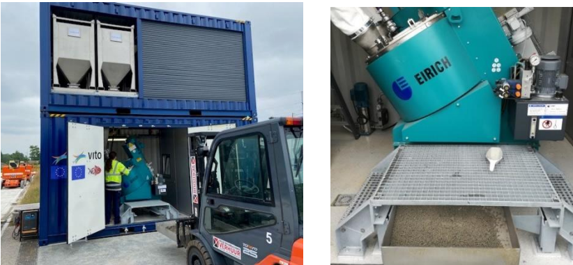
Figure 4: Granulation and concrete production pilot at VITO (left) focused image of the Eirich mixer after granulation (right).
