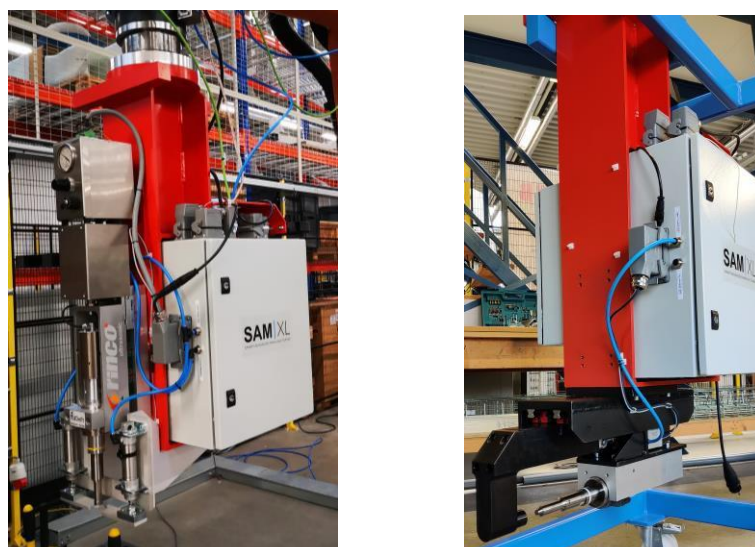
Figure 2: Robotic End-Effector for Clip-To-Skin (left) and Clip-To-Frame (right) Ultrasonic Welding
