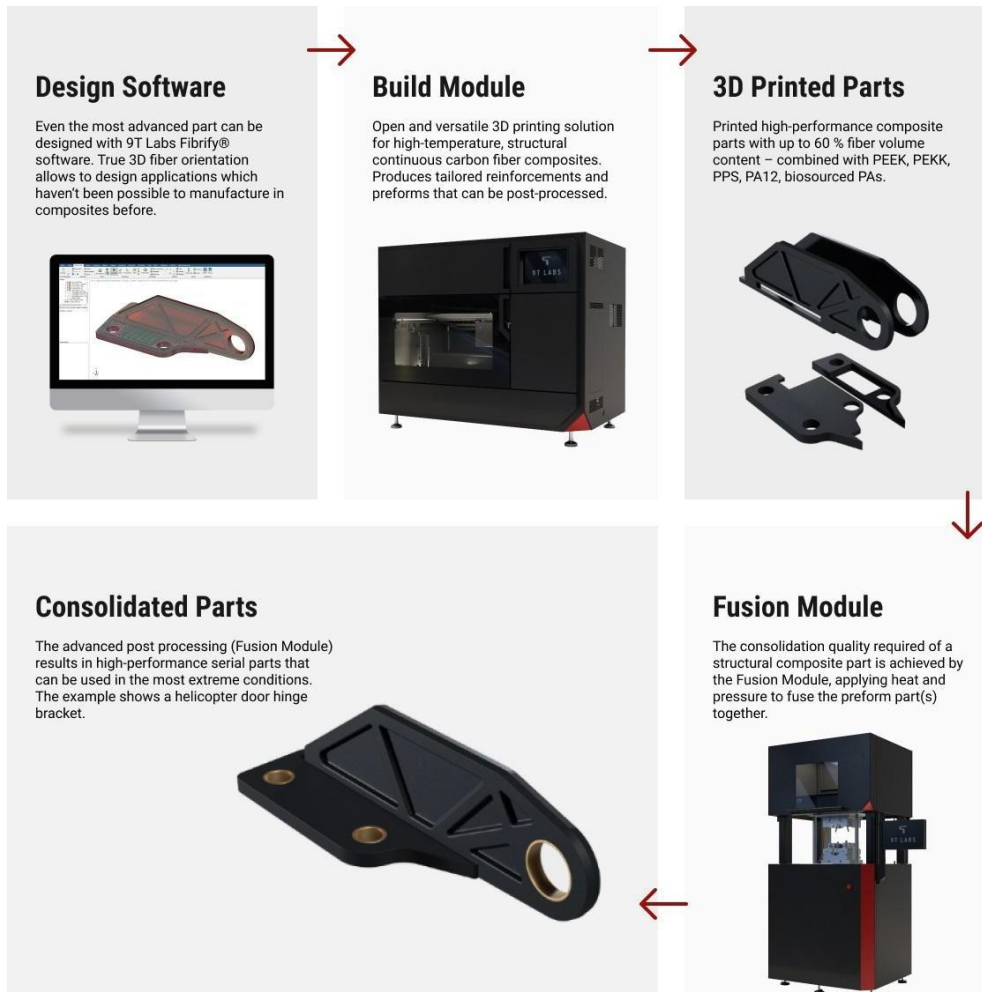
Figure 1. Additive fusion technology consists of advanced design software, a 3D printer that produces (near-)net-shape preforms, and a compact compression press equipped with matched metal dies in which preforms are heated, shaped, and consolidated.
