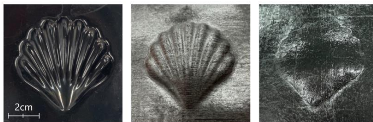
Figure 2: Shell mould (left) and formed preforms; aligned fibre (centre) and continuous fibre (right).
