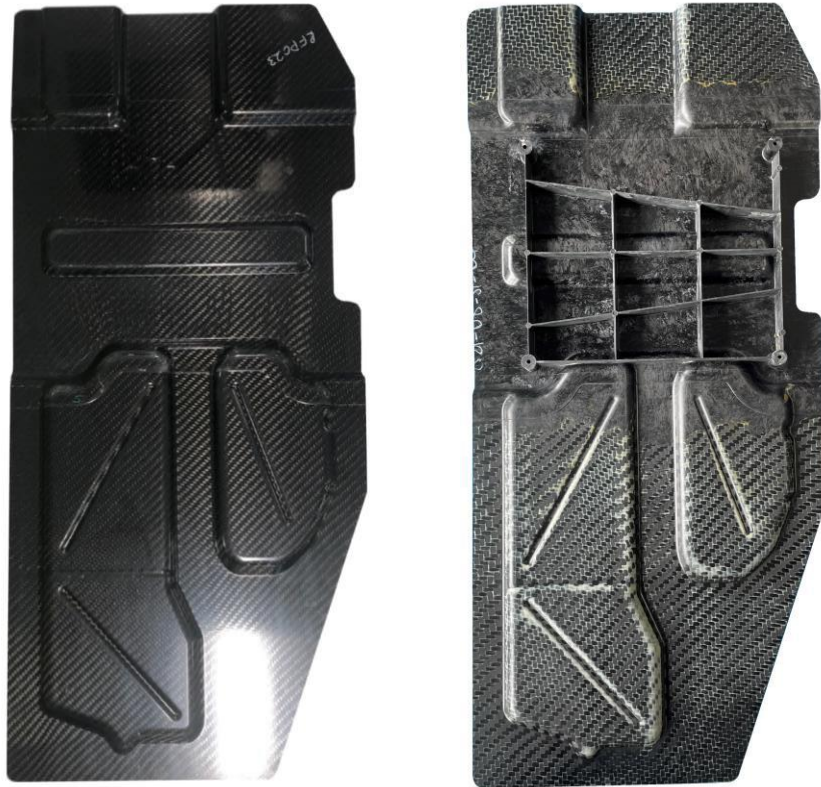
Figure 1: Prototype floor pan produced on InterCOMP (left) and CADFEC (right).
