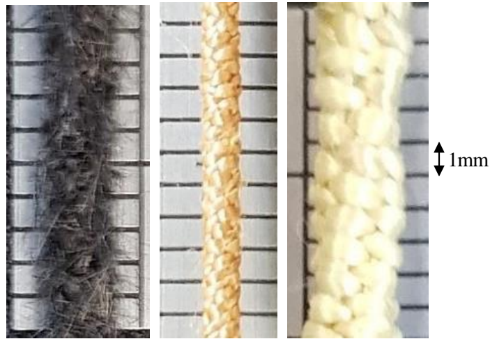
Figure 3: Circular cross section carbon fibre-epoxy rods overbraided with Toray T300 carbon (left), Teijin high modulus Zylon (centre) and Teijin Twaron 2200 aramid (right).
