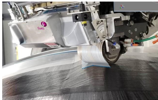
Figure 1: Scanning head mounted on a Viper 4000 Automated Fibre Placement Machine
