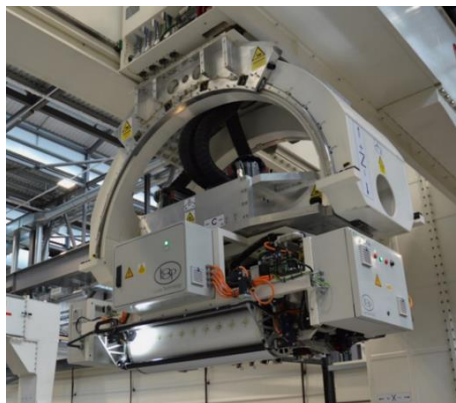
Figure 3. A 1.3 m FibreROLL system, gantry mounted
