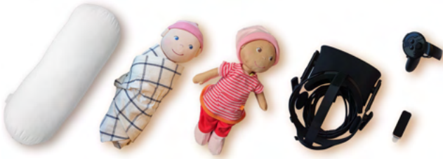
Figure 4: (From left to right) Physical representations of the baby, VR head mounted device and sensors for hands and motion tracking
