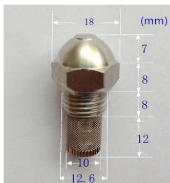
Fig. 1. The experimental nozzle geometry.
