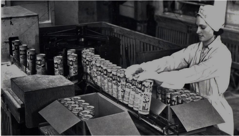
Figure 2 —Lever Brothers, Port Sunlight Works (near Liverpool, UK), Vim packing department—probably at the end of the 1930s. The silica flour is mixed with powdered soda ash, soap, and sometimes other substances, either with a shovel, or in a mixing machine. Filling the cartons may also be done by hand, or by mechanical fillers; the lids are then placed and fixed by a machine.” 19,20
