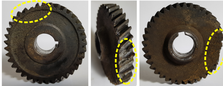
Figure 13: The gear before the experiment started and after the experiment was completed are presented in Figures 13(a) and 13(b) respectively. The damaged regions of the gear are clearly highlighted in Figure 13(b).
