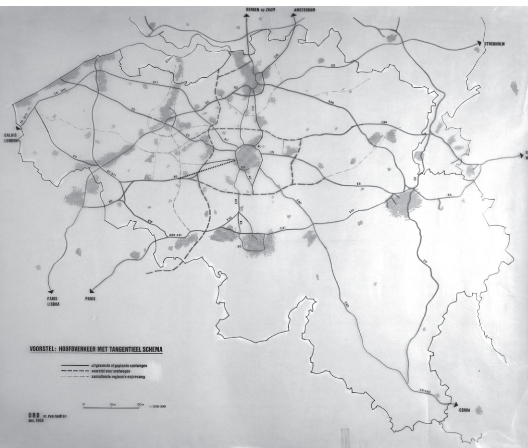
Figure 6: design for a tangential high way system around Brussels superimposed on the radio-concentric system. M. Van Naelten, 1969. Source: IISRO Archives, KULeuven
