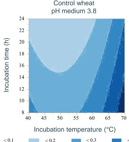
Phytate content in wheat hydrothermally processed at 50 °C, pH 3.8 for 8 h is predicted and verified to decrease from 0.96% initial dm to 0.17% initial dm as a result of optimal endogenous phytase action
