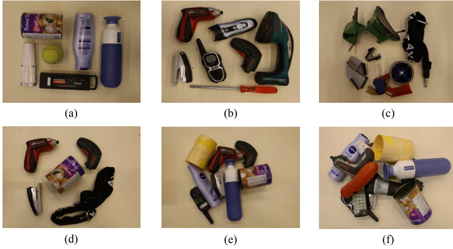
Fig. 11 Examples for the objects' complexities and distributions. (a) A set of objects with basic shapes. (b) A set of objects with regular shapes. (c) A set of objects with complex shapes. (d) A set of objects in independent distribution. (e) A set of objects in single-layer contact. (f) A set of objects in multi-layer contact.
