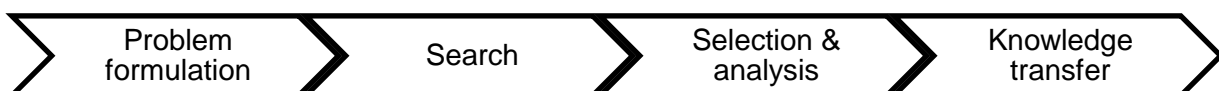
Figure 1: The phases of the systematic bio-inspired design process as identified by Vandevenne et al. (2015).
