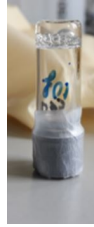
Figure A.1: Vial turning technique for a batch of successfully grafted fd-pnipam.
