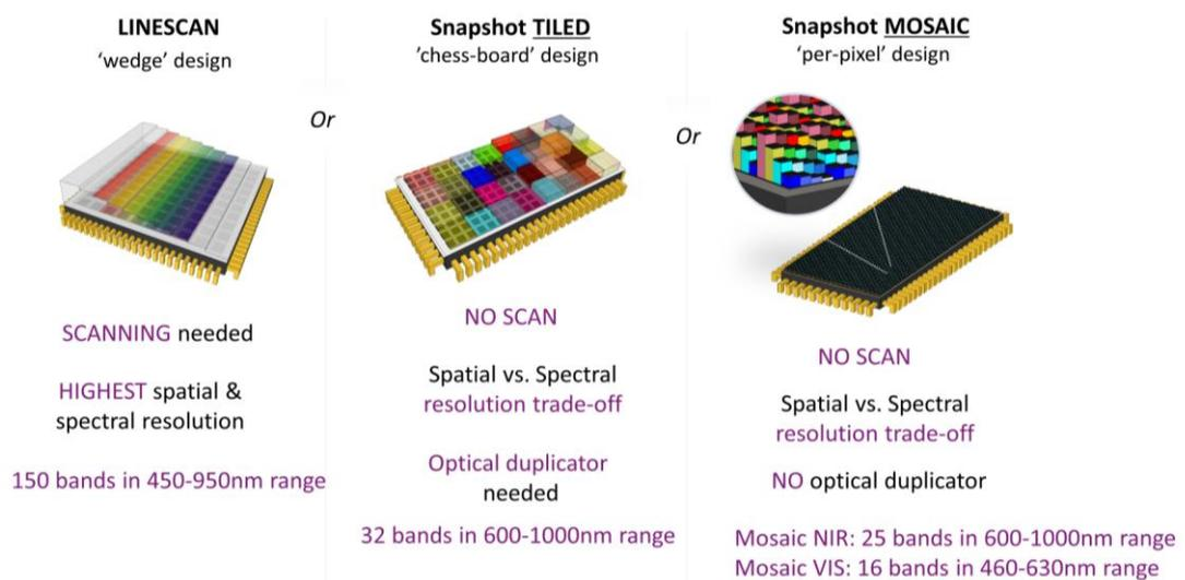
Figure 1-13: Illustration of the different hyperspectral sensors developed by IMEC with their spatial and spectral characteristics – Image Courtesy of Imec.
