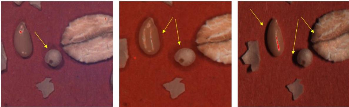
Figure 4-14: Illustration of the impact of the spatial distribution of illumination: Halogen (left), Tunable LED system (middle), Fixed LED system semi-diffuse (right). The arrows indicate the seed shadow locations.
