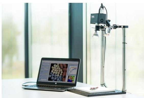
Figure 3-2: Imed Snapscan System with Snapscan camera USB-connected to laptop
