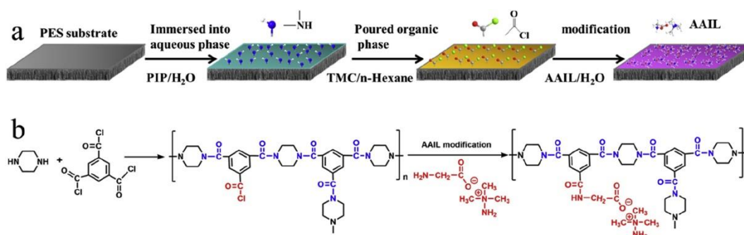
Figure 1.9 (a) Schematic diagram of an AAIL modified NF membrane, and (b) the reaction formula [99].
