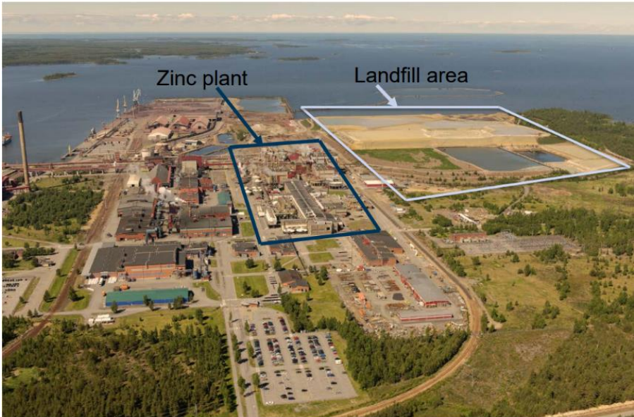
Figure 1.5: Europe's second largest zinc production plant and the jarosite landfill area of Boliden in Kokkola, Finland. Photo available online by courtesy of Boliden ( http://prometia.eu/wp-content/uploads/2014/02/05_Salminen_Boliden.pdf ).
