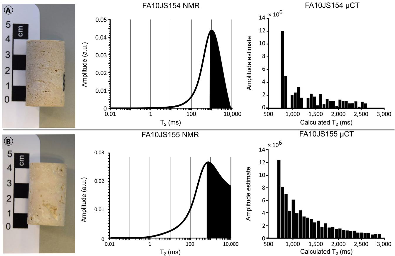
**FIGURE 13** Plug samples and their respective NMR and XCT  $T_2$  distributions. (A) FA10JS154 with XCT calculated  $T_2$  values from 800 ms up to 2,600 ms. (B) FA10JS155, with a NMR distribution with a strong shoulder towards 10,000 ms. XCT  $T_2$ -times up to 3,000 ms were calculated
