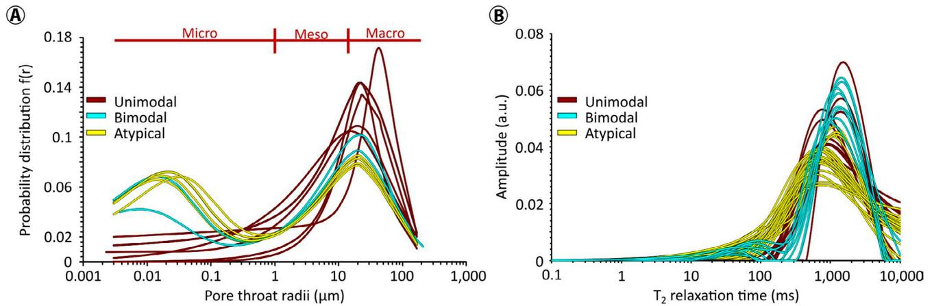
**FIGURE 7** (A) MICP pore size distributions. The samples have an unimodal or bimodal distribution. The main peak of the distributions is found between 1 and 200  $\mu\text{m}$ , bimodal samples have a secondary peak, which is located between 3 nm (the lower limit of the technique) and 1  $\mu\text{m}$ . (B) NMR  $T_2$  distributions. Unimodal, bimodal and atypical (bimodal in MICP, but not in NMR) NMR curves are observed
