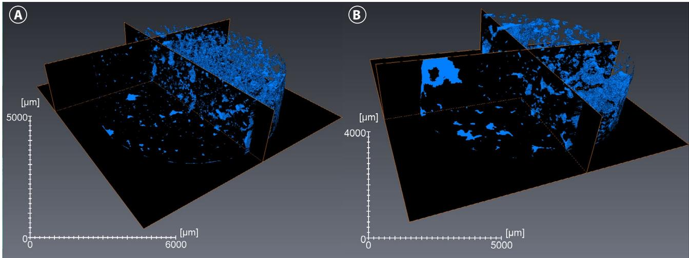
**FIGURE 14** Orthogonal slices and partially volume rendered pore networks. (A) Sample FA10JS150 with small pores in a pore distribution with typically  $800 < T_2 < 2,600$  ms. (B) Sample FA10JS047 with fewer, but large pores, typical for calculated  $T_2$  values reaching up to 3,000 ms
