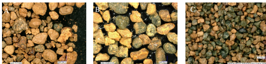
Figure A4.2 Removal of the Fe-coating with water on a strongly naturally weathered sample (W11) in two washing steps. With A) the unwashed sample, B) after one rinsing and C) after a second washing. The remaining oxidised grains are assumed fully oxidised. In the subsurface glauconite sands there is very little difference before and after washing.
